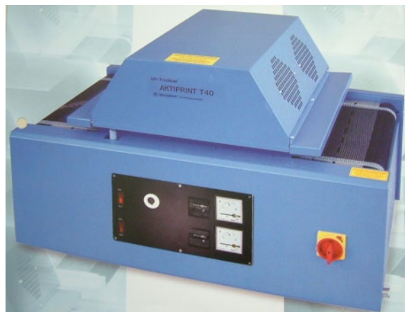
UV heater with conveyor belt
