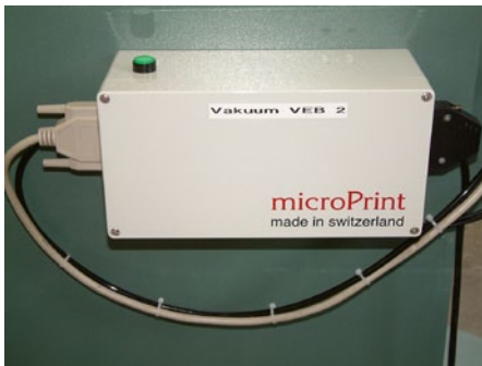
Vacuum Retaining and Compressed Air Rejection Unit VEB2
