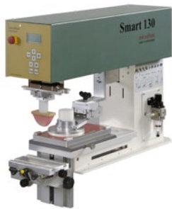
Simple pad printing machine with pneumatic drive
