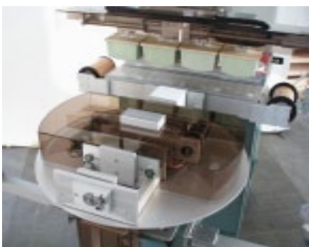
Multi-color printing machine MS 500 with pad shifter
