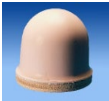
Round pad with round print area. Most suited for printing of round objects
