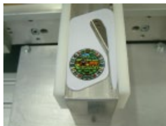
Multi-color printing machine MS 250 with pad shifter
