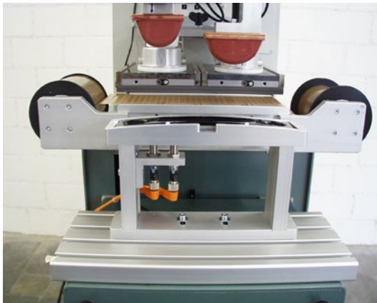
Transportation element not extended
