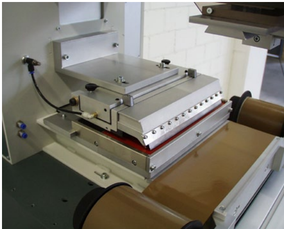
Pad cleaning with closed ink system
